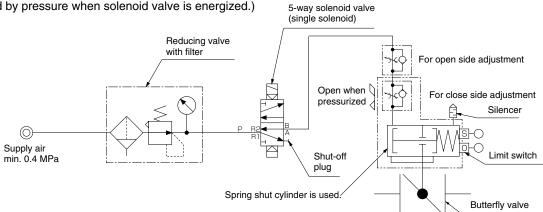
2 Butterfly valve opens when power supply falls. (Closed by pressure when solenoid valve is energized.) Butterfly valve opens when air supply falls. (Closed by pressure when solenoid valve is energized.)
