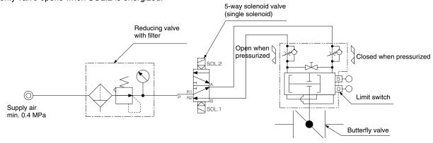
→Once SOL.1 is energized, the condition is maintained even after it is de-energized unless SOL.2 is energized.
